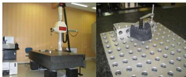
**Figure 2:** right: CMM, left: A cast fixed in the machine
