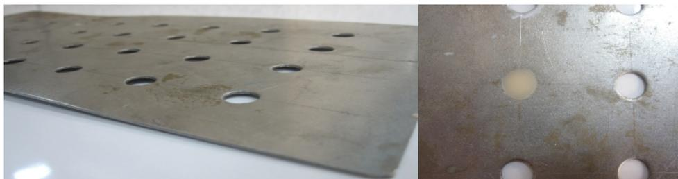
**Figure 1:** Disc-shaped moulds for fabrication of solubility testing specimens
