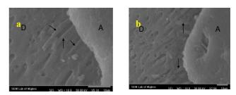
Figure 1: Scanning electron micrograph of filled and unfilled SE Bond. a) low-magnification representation of bonding area in unfilled adhesive {(D) dentin, (A) adhesive} Arrows indicate resin tags. b) the same magnification representing bonding area in filled adhesive
