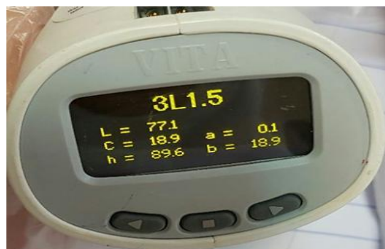
Figure 3. Color evaluation by using the VITA Easyshade® spectrophotometric device
