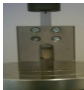
Fig 2. Placement of the prepared sample in Zwick machine
