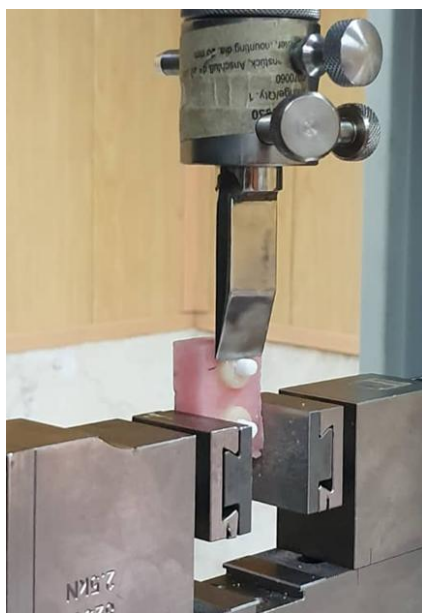
Figure 2. Sample placed in a universal testing machine for measurement of shear bond strength
