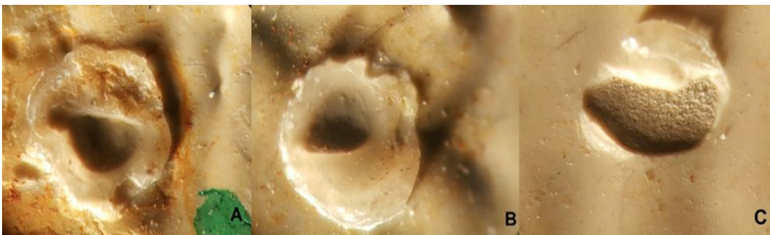
Figure 3. Mixed failure type in Co-Cr (A), PEEK (B), and zirconia (C) groups
