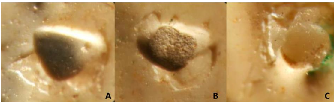
Figure 2. Adhesive failure type in Co-Cr (A), PEEK (B), and zirconia (C) groups
