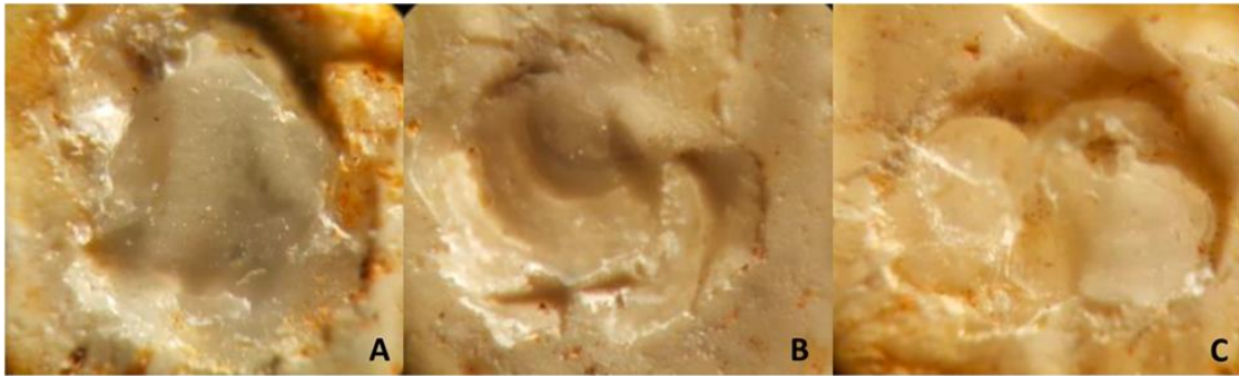
Figure 1. Cohesive failure type in Co-Cr (A), PEEK (B), and zirconia (C) groups
