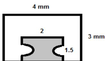
**Figure 2.** Schematic view of the cross section of specimens in group 3
