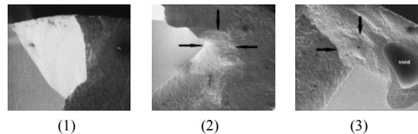
**Figure 7.** Shows the fracture surface of a group 3 specimen. It appears that the fracture started at the external surface of the specimen, propagated towards the interface and spread from there (white arrows)
