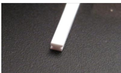
**Figure 3.** Trenched zirconia bar
