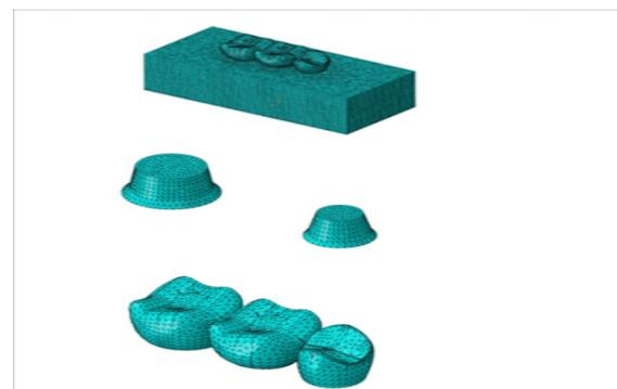
**Figure 1.** The shape and geometry of the meshed three-unit FPD model Model/Luting cement layer/ Supra-structure
