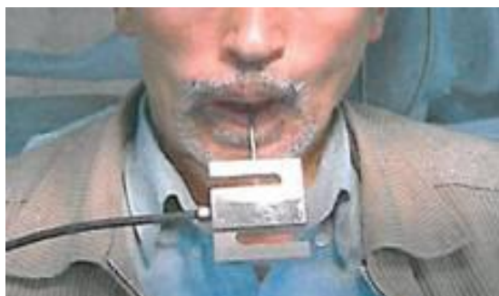
Figure 2. Measuring the load required for dislodgment of the maxillary denture base
