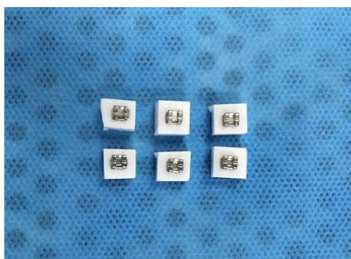
Figure 1. Bracket bonded to zirconia samples
