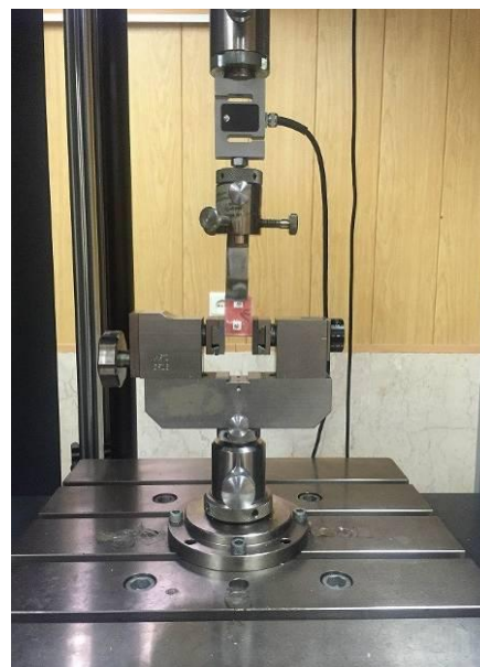
Figure 2. Sample in universal testing machine for SBS test
