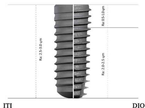
Figure 1. Comparing the shape and surface roughness of implants
