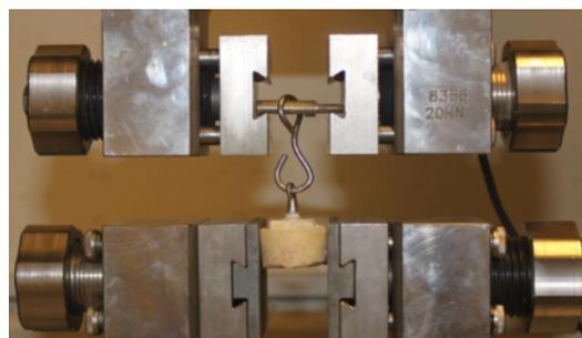
**Figure 2.** Measurement of tensile strength
