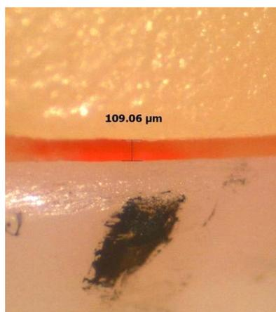
**Figure 4.** Gap measurement using stereomicroscope at  $\times 35$  magnification.
